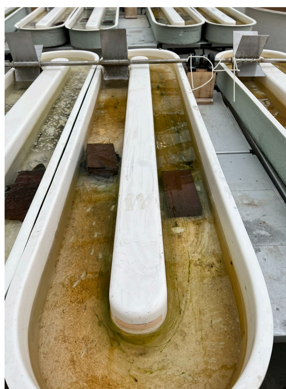
Figure 5. Stream D4 with no salt and low nutrient treatments in Week 4. BioChar bags were submerged and held under bricks to prevent movement.
