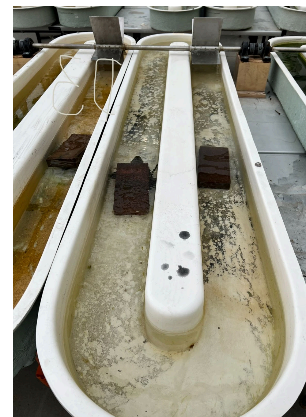
Figure 7. Stream D3 with salt present and no nutrient treatments in Week 4. BioChar bags were submerged and held under bricks to prevent movement.
