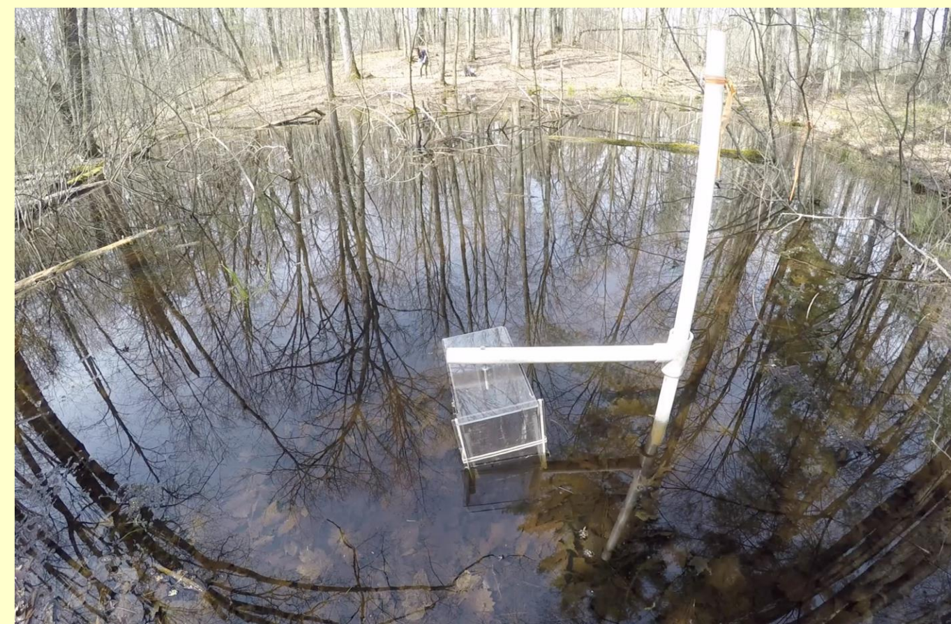
Figure 2a: SAT placed in the wetland for collecting macroinvertebrates. Traps would remain in position for 24 hours before being collected.
