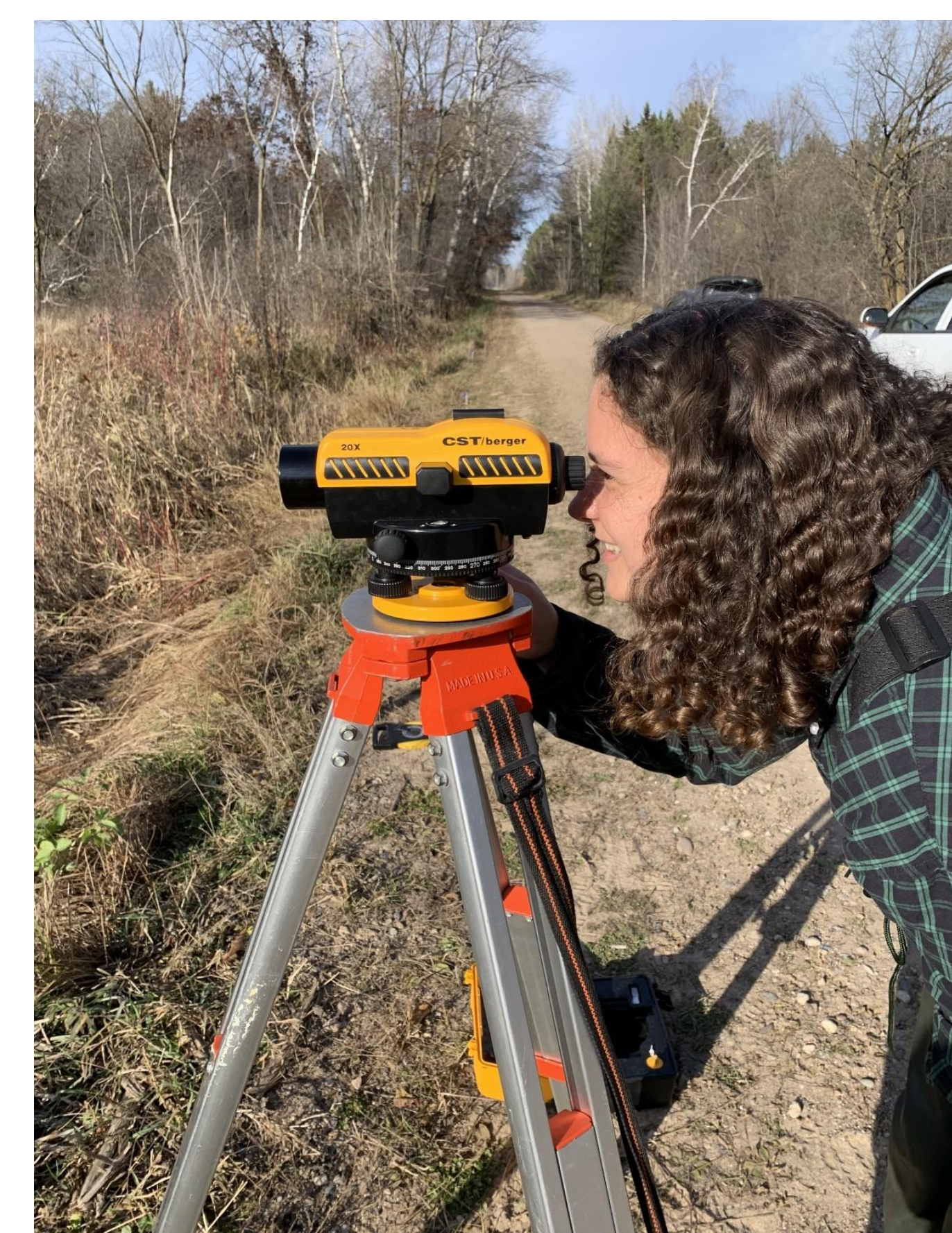
Figure 4. Using a dumpy level to measure elevation in the wetland.
