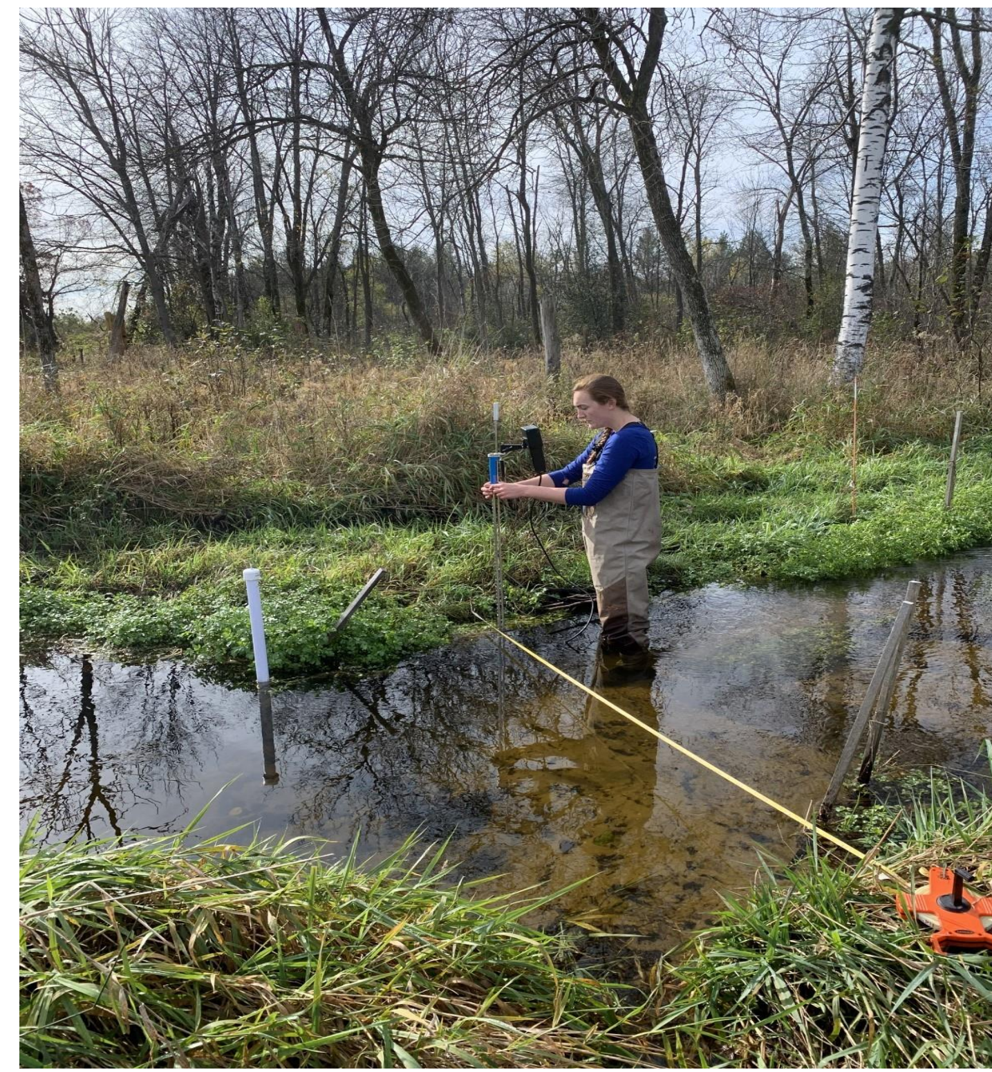
Figure 2. Using a Flow Tracker to take discharge measurements near the upstream stilling well.
