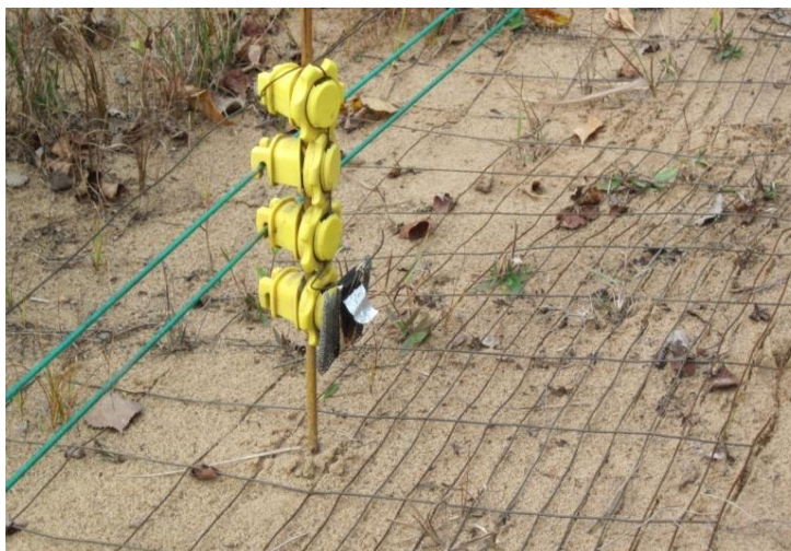
Figure 2. Fencing scheme: hot line at 10 inches above substrate, wire-core clotheslines at 6 and 8 inches, bait packet, lightweight wire fence grounding screen (here, without design enhancements, see text, pg. 4).
